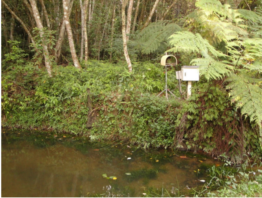
Figure 2. Lienhuachih Frog Pond: Three species of frog live in this pond. The field microphone is on the tripod on the left and the field computer is in the box on the right.
