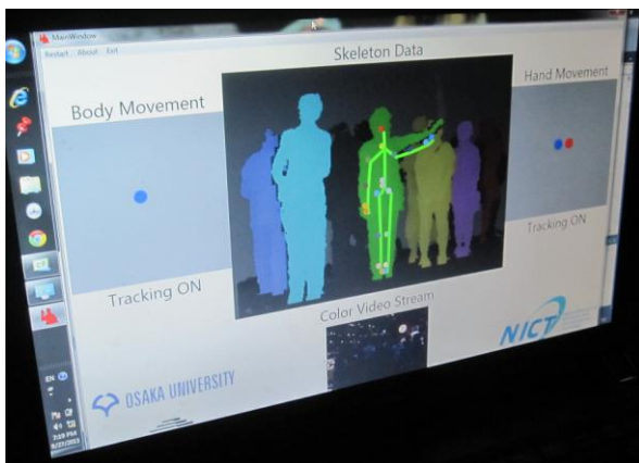
Figure 6: Interface of my Kinect Application. Note the person tracked is the user with the skeleton displayed, ignoring all others tracked.
