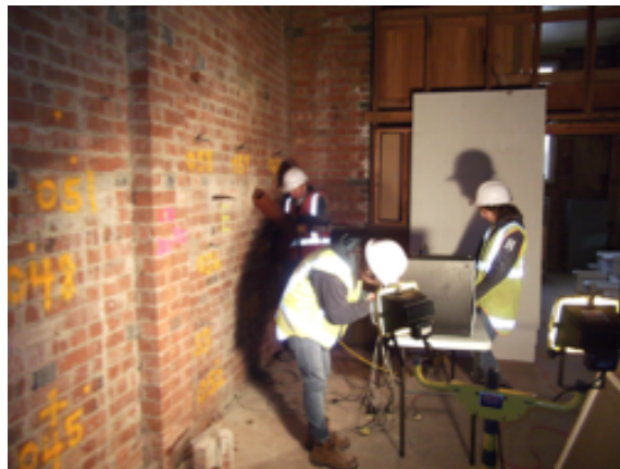
Figure 2: Overall anchor pull-out testing set up including the on site monitor and computer to record the force and displacement results.
